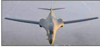
U.S. Air Force photo by Senior Airman Rebeca M. Luguin A B-1B Lancer performs a low-level fly-by for troops deployed for Operation Enduring Freedom Oct. 27. The B-1B's three internal weapons bays can accommodate up to 84 MK-82 general purpose bombs or MK-62 naval mines, 30 CBU-87/89 cluster munitions or CBU-97 Sensor Fused Weapons.
