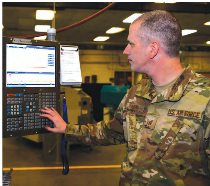
Left, Tech Sgt. Robert Burns, 56th Equipment Maintenance Squadron aircraft metals technology noncommissioned officer in charge, inputs a command into a 5-axis computer numerical control machine, February 6, at Luke Air Force Base. Metals technology provides machining and welding operations for aircraft and support equipment across the base. Right, Airman 1st Class Taylor Frost, 56th Equipment Maintenance Squadron aircraft metals technology apprentice, shaves down an ammunition shell. Airmen assigned to the 56th EMS metals technology shop provide disciplined and innovative maintenance approaches to support the fifth generation and legacy aircraft housed at Luke AFB. (U.S. Air Force photo by Airman 1st Class Zoie Rider)
