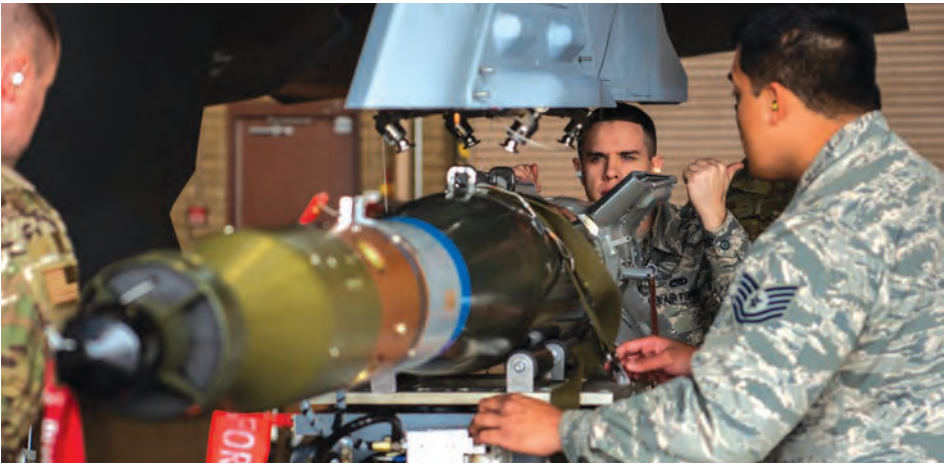
Senior Airman Levi Aydt, 56th Component Maintenance Squadron load crew member, directs the jammer driver to position dummy munitions on an external pylon. The F-35A Lightning II can have external pylons installed for additional munitions while in combat. (U.S. Air Force photo by Airman 1st Class Aspen Reid)
